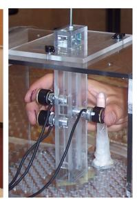
Lucius interface and acquisition system of biological signals (Left panel). Application being used with balance and EMG equipment (Middle panel) and interface created for testing of multi-finger coordination and force production (Right panel). The system can also integrate any other instruments (thermocouples, encephalography, electrocardiography, etc.) and produce biofeedback to patients and researchers. Analytical system is customizable for future clinical use and systems are mobile.
